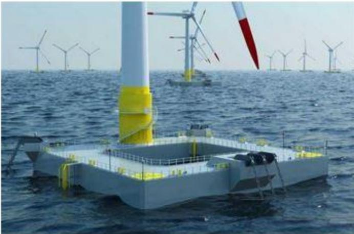
Floatgen first... Installation is expected next year of a Floatgen demonstrator using Ideol's "damping pool" floater
